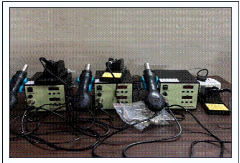
Hot Air Blower with Soldering Iron
